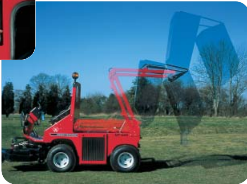
'Collect' or 'Discharge' grass cuttings by moving a convenient lever
