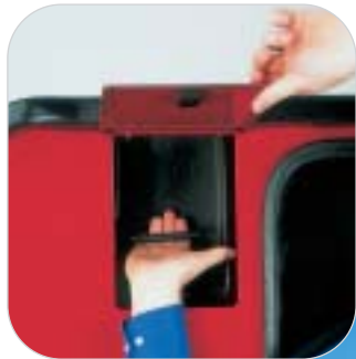
'Collect' or 'Discharge' grass cuttings by moving a convenient lever
